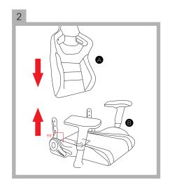
Remove the M8 screws from the seat back/top. Place the seat back/top onto the seat base between the metal hinges.
