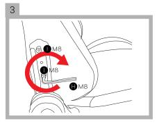
Use an M8 Allen key to fix the seat back/ top onto the seat base metal hinges, using the same M8 screws.
