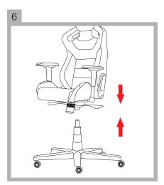
Insert the gas lift piston into the notch of the gas lift regulator underneath the seat. No screws needed, balance the seat and it will click in place. Gently apply pressure.
