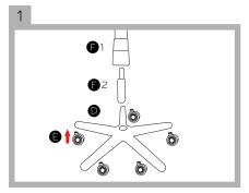
Install the wheels, gas lift piston and the piston cover onto the star base. These parts are easy to install.
